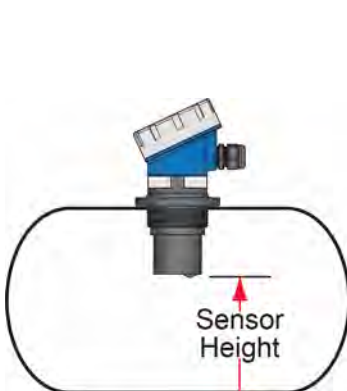
Simple Horizontal Tank
